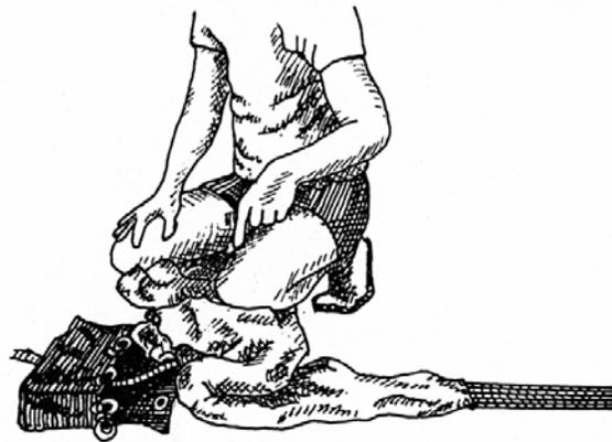
13) Push the canopy into the bag. Make sure that you keep the canopy in a bundle as you go. Push any remaining parts of the canopy neatly into the bag.
