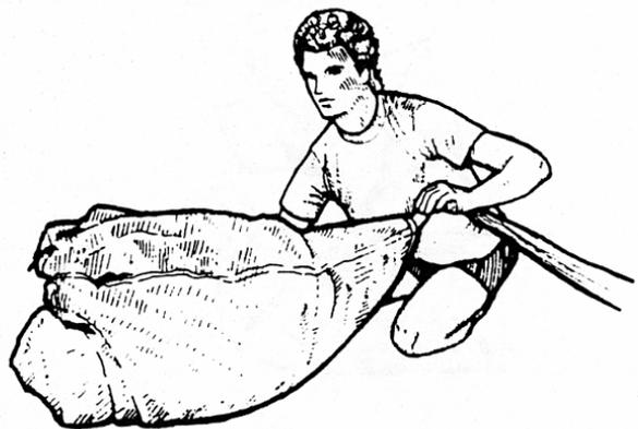
9) Push the lateral canopy parts together and under the bundle. Beginning at the slider, kneel on the canopy and form a “cocoon” the width of the deployment bag.
