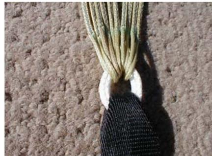
6) Rotate the link so that the knotted portion is hidden inside the riser. Finally, pull the riser and suspension lines away from each other to tighten the connector link. It is important that the locking section of the link remain inside the riser, so for the first several pack jobs check for this. After a few jumps the link will take a "set" and have no tendency to rotate.
